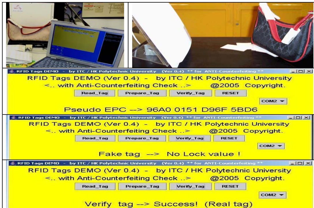
Fig 7. Top left: Equipment setting (Notebook PC with anti-counterfeit checking application, RFID antenna, RFID reader, and a tag embedded inside a bag). Top right: Distance setting between a RFID antenna and a bag (about 30cm). Second row: Anti-counterfeit checking application reads the bag and displays the encrypted EPC code (pseudo-EPC) of the embedded tag. Third row: If the tag is not genuine, the checking application will show that this is a fake tag with possible reason. Bottom row: If the tag verification is done properly, the tag inside the bag is genuine, and the apparel product is said to be genuine.
