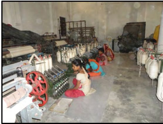
Figure 10: Spinning using NMC charkha with 8 spindles in the unit (Moradabad and Jind)
