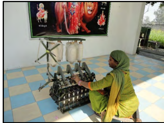
Figure 10: Spinning using NMC charkha with 8 spindles in the unit (Moradabad and Jind)
