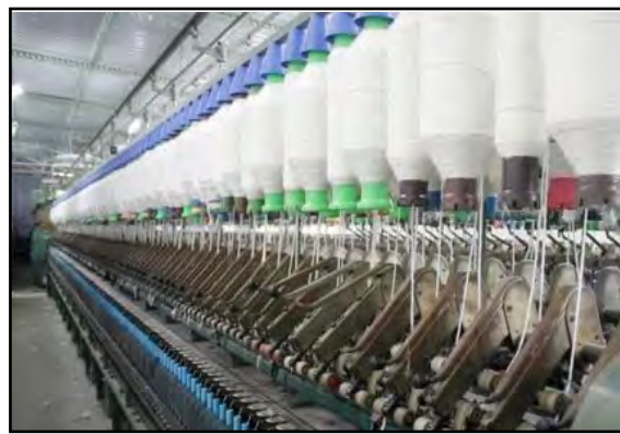
Figure 2: Mill spinning of yarn used for handloom and powerloom
