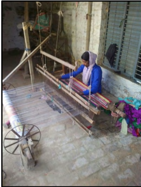
Figure 19 and 20: Weaving done on pit loom
