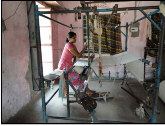
Figure 17: Weaving done on traditional (frame loom)
