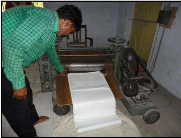
Figure 25: Pressing and folding of fabric
