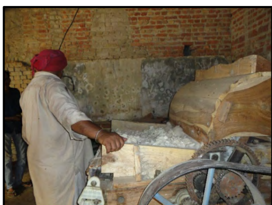
Figure 4: Cotton placed on the top of carding machine
