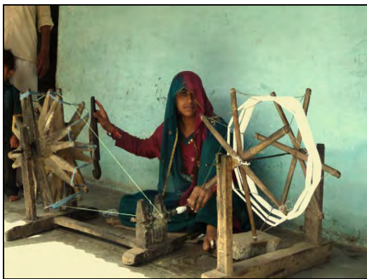
Figure 1: Hand spinning of yarn used for khadi
