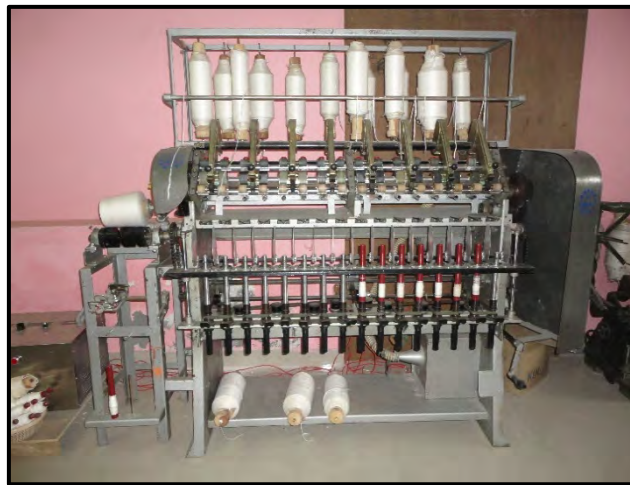
Figure 11: Spinning using solar charkha (Jind)
