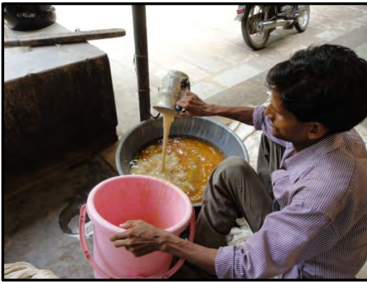
Figure 12: Starch was applied on yarn hanks
