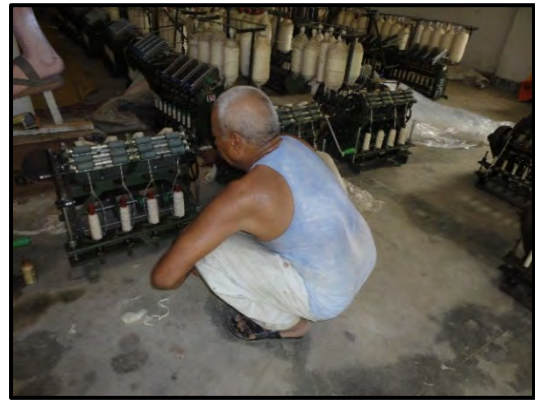
Figure 6 and 7: Working of belni machine by rotating handle-Avadh Yuva Kalyan Gramodhyog Sansthan, Moradabad (Uttar Pradesh), June 2018
