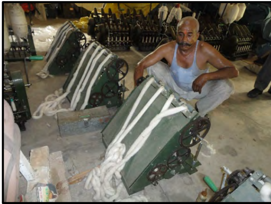
Figure 6 and 7: Working of belni machine by rotating handle-Avadh Yuva Kalyan Gramodhyog Sansthan, Moradabad (Uttar Pradesh), June 2018
