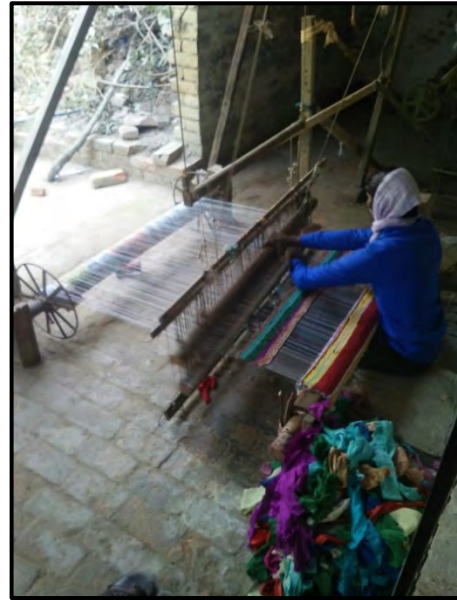
Figure 19 and 20: Weaving done on pit loom
