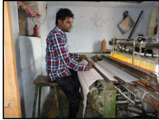
Figure 17: Weaving done on semi-automatic peddle loom
