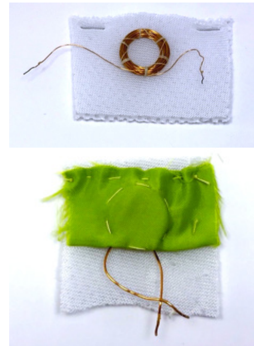
Figure 6: Electromagnet (Left: Without magnet. Right With magnet)
