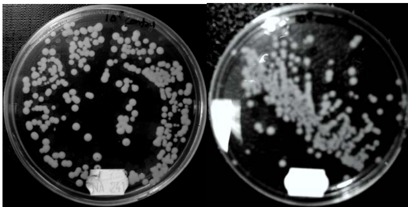
Figure 8. Control (untreated) for woven and knitted samples showing bacterial growth on agar plate
