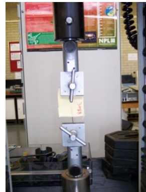
Fig. 6. Woven sample held in Instron tensile test machine part way through extraction.
