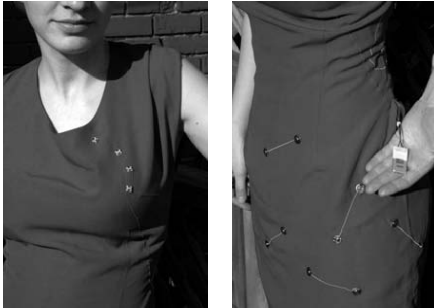
Figure 2. The electronic circuit is distributed over the body of the dress. The four LEDs provide the visual output. The power source consists of a lithium polymer rechargeable battery, held in a custom-made pocket at the waist. The interactive interface consists of the pairs of snaps that act as switches and allow us to close the circuit (turn the LEDs on) by connecting to another dress
