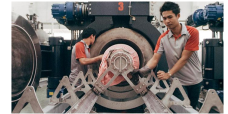
Fig. 1 Waterless dyeing from the Yeh Group, featured in The Next Black (The Next Black 2014)
