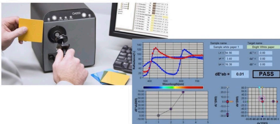
Figure 20. Spectrophotometric Colour-Matching System used in Textile Industry
