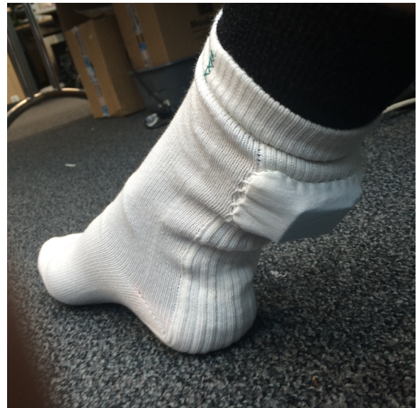
Figure 3: Temperature sensing socks developed for wear trial
