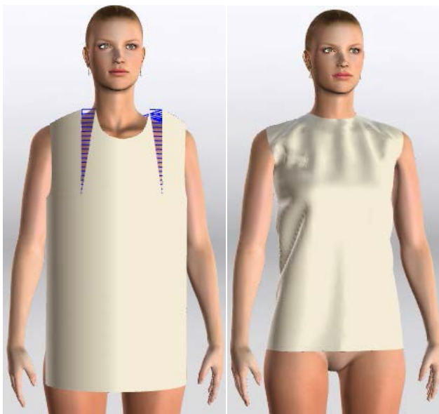
Figure 6. Pattern Placement on Avatar (left) and Virtual Blouse after Simulation
