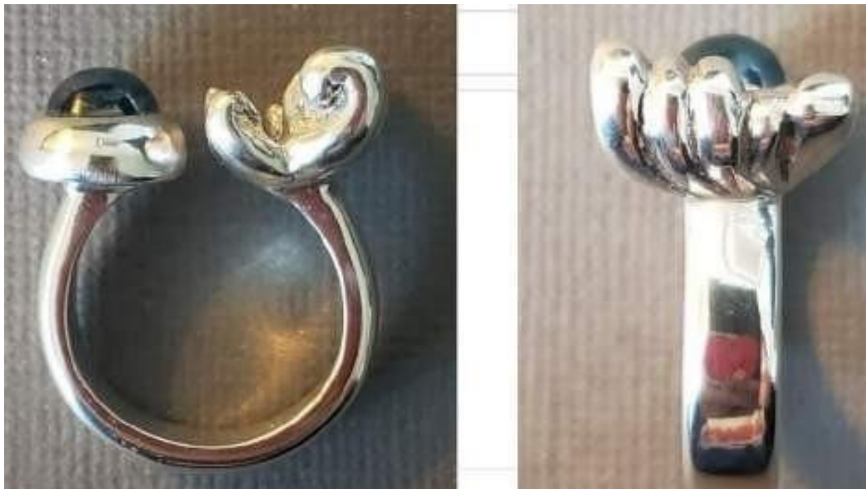
Figure 12. Rings from the second semester. The assignment was to create a ring that features a bezel-less setting. This ring embodies all the learning goals from the previous one, with the added tasks of learning to clean up and polish the casting, and setting the stone. Students were taught to make their own setting tools in steel for this project.
