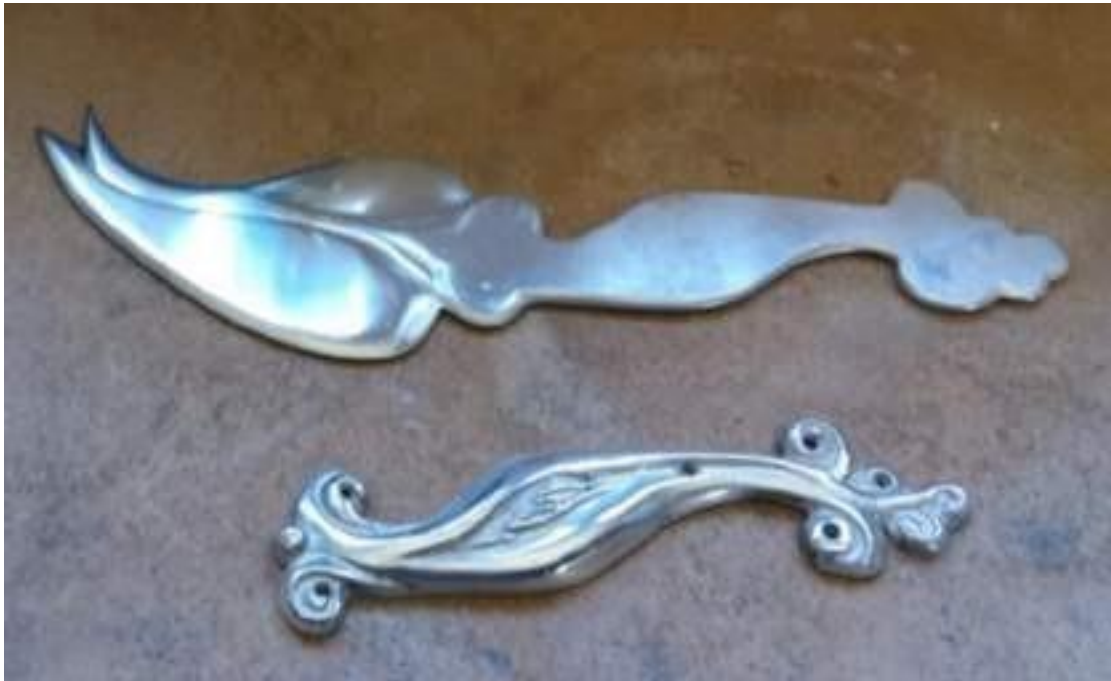
Figure 15. The cheese knife parts are ready for assembly. The three-dimensional effect on the blade was created by filing and polishing.
