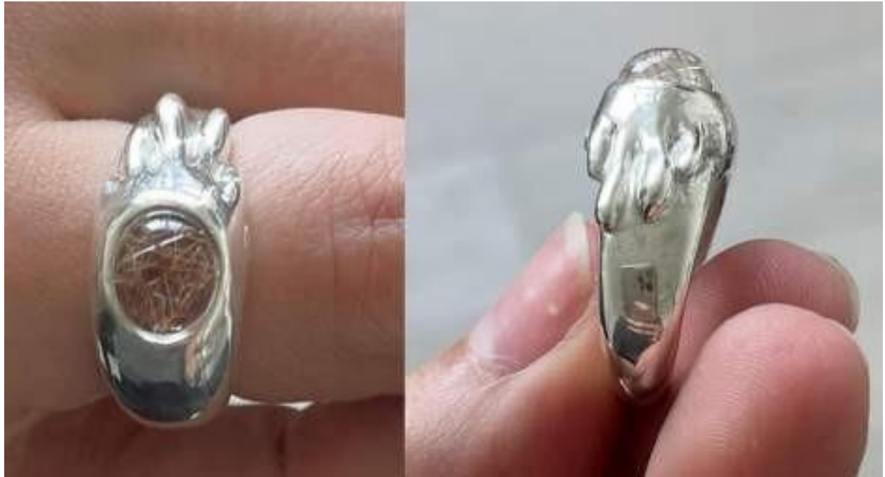
Figure 12. Rings from the second semester. The assignment was to create a ring that features a bezel-less setting. This ring embodies all the learning goals from the previous one, with the added tasks of learning to clean up and polish the casting, and setting the stone. Students were taught to make their own setting tools in steel for this project.
