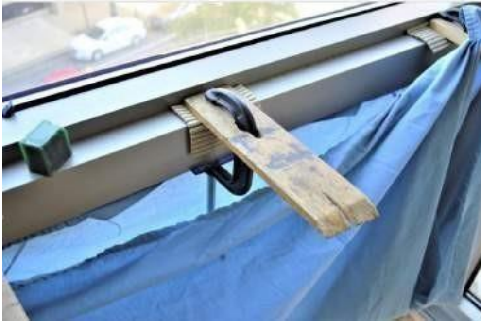
Figure 2. This is a workspace created at home using the ledge of a window sill. The blue pillowcase is positioned to catch wax filings. One of the most important things we teach in our curriculum is working safely. We teach the importance of bench height in ergonomics, good light and ventilation, as well as the necessity of keeping the place clean to avoid cross contamination of working materials with living spaces. The positioning of Smartphones over each student's workspace allowed us to monitor safe working—and to correct problems instantly before bad working habits could form.
