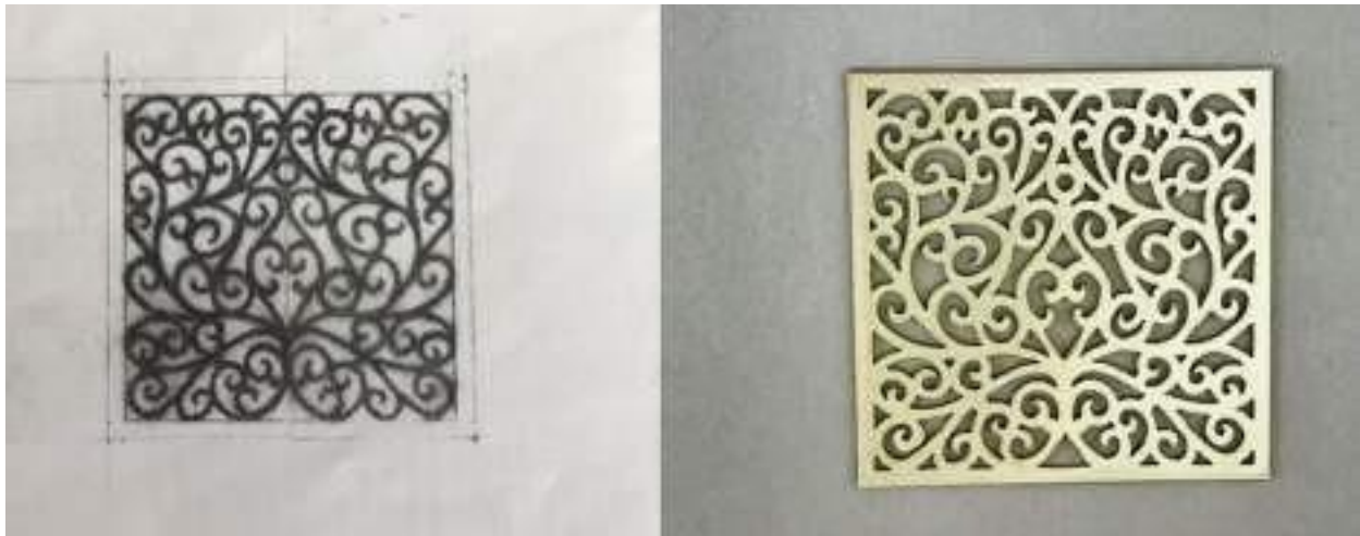
Figure 6. This is the teaching example Professor Teratani made for the first project. The thickness of the brass is 18 gauge--one millimeter. This project teaches precision and confidence with the jeweller's saw. Filing to correct wavy cuts was not permitted. Students were required to hand in their photos of their original design and their finished work for comparison and accuracy.
