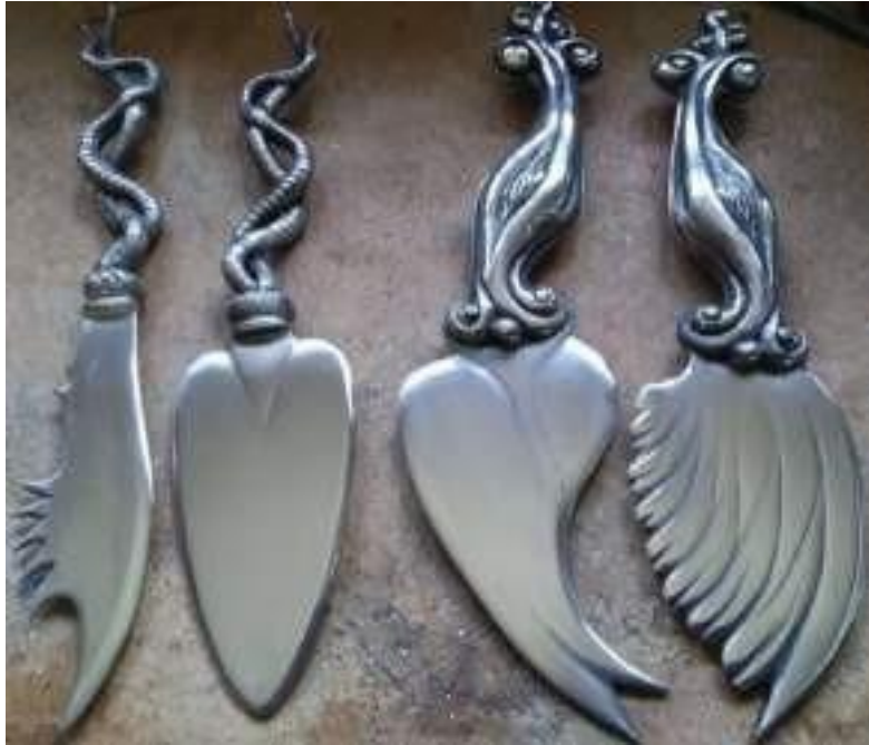
Figure 14. These are teaching examples created by Wendy Yothers. The handles were carved, cast and riveted onto the knife.
