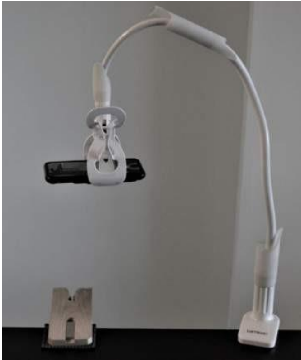
Figure 1. Gooseneck tripod with Smartphone positioned over the student's bench pin
