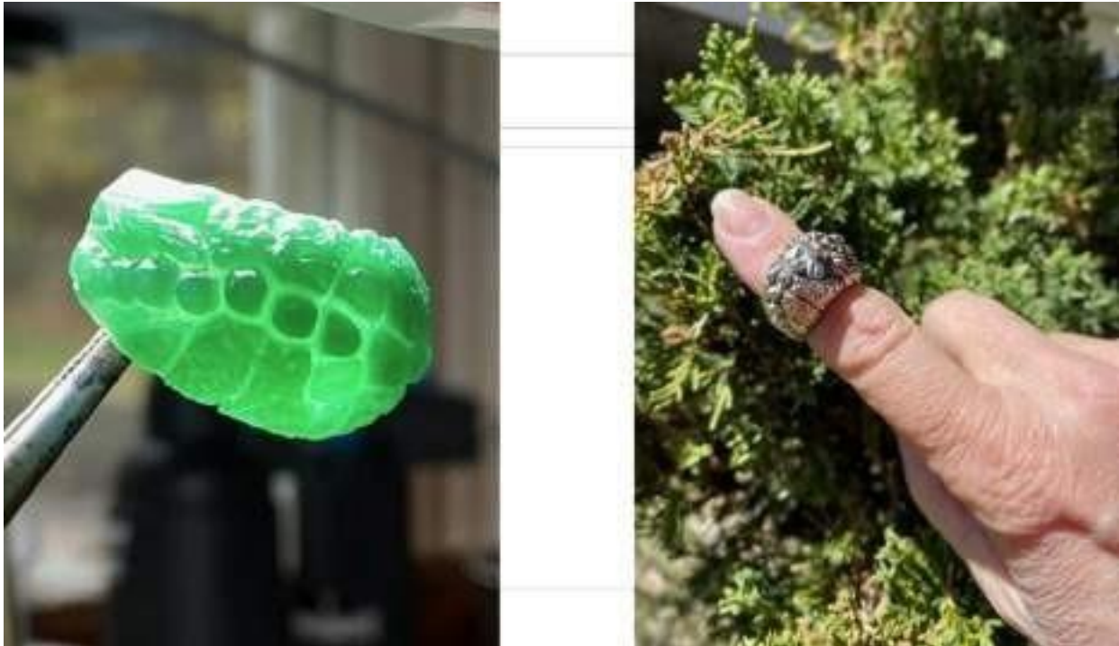
Figure 10. These two photos illustrate the ring in progress and finished. Light is used as a tool for checking the thickness of the carved wax. Darker areas are thickest, and must be hollowed out to a single millimeter before the ring can be cost-effectively cast in precious metal.
