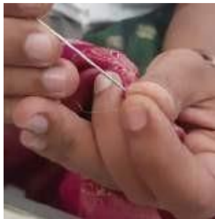
Figure 9. The number of ply is checked in one warp zari thread (In this there were 6 plys)
