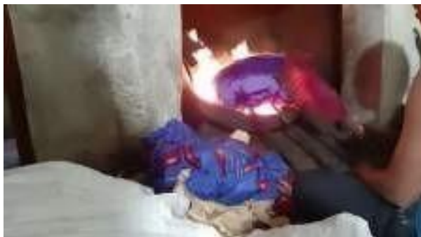
Figure10. The process of saree burnt into ashes to extract gold and silver
