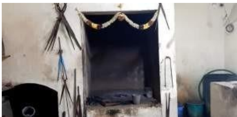
Figure 11. The traditional stove or Aduppu to heat the ashes which contains gold and silver
